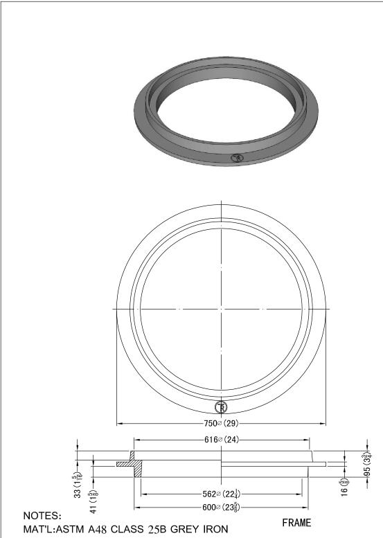
FINISH:BITUMINOUS DIP LOADING:HIGHWAY LOADING
